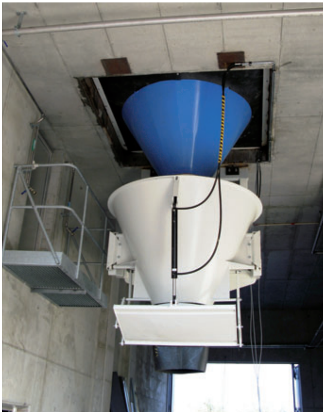
The special bin is for loading all types of trucks. The low one is for 12m3 trucks that are used in the mine, and the normal one is for normal truck mixers for the street.
